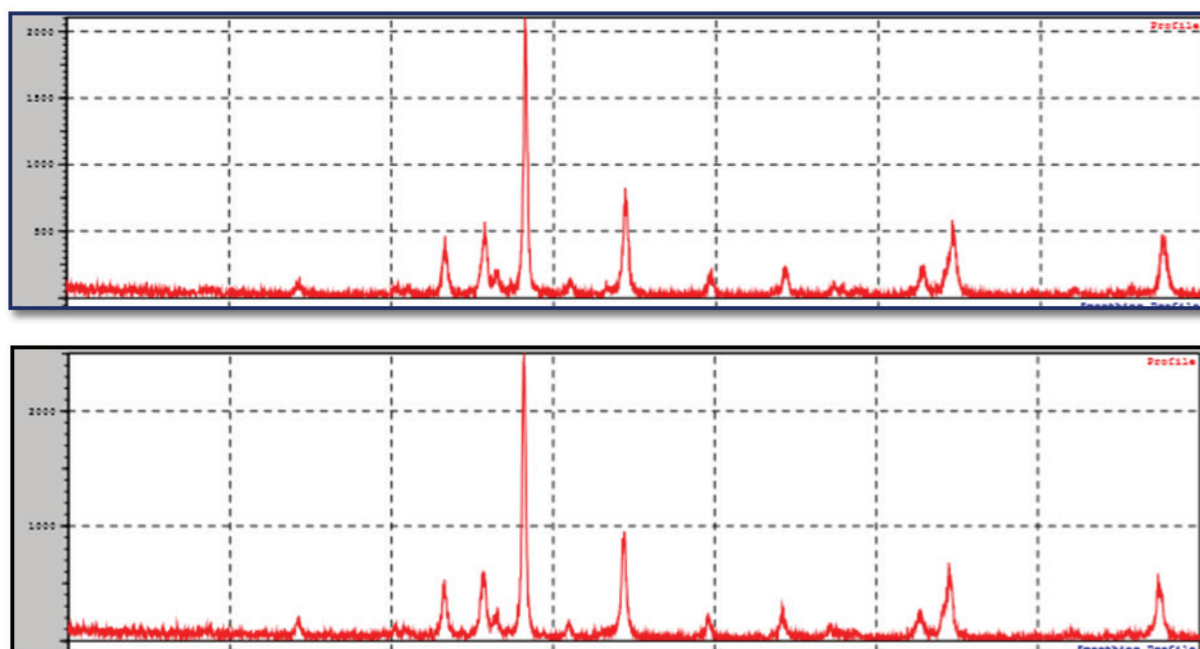
Fig 5. X-ray diffraction spectrum of spinel.
