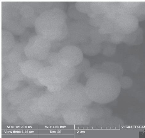
**Figure 2. SEM of chitosan-alginate nanoparticles in view-field 6,35 µm**
