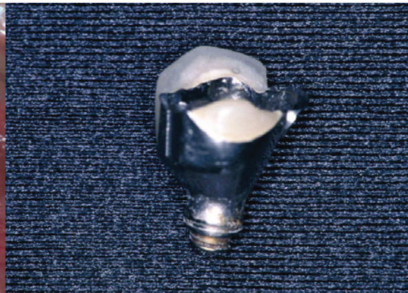
Fig 4: Implant restoration together with fractured implant component [1]
