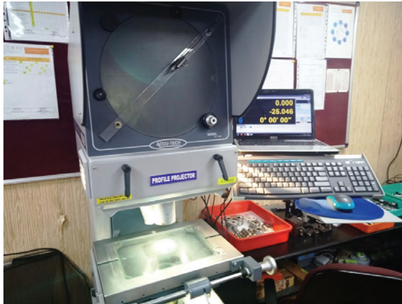
Figure 4 : Determining dimensional accuracy of impression material using vertical profile projector
