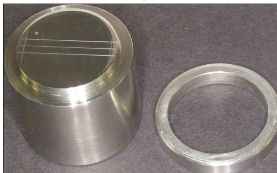
Figure 2 : Stainless steel die
