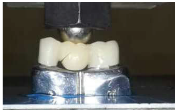
Figure 5. Fracture of the bridge after load application.
