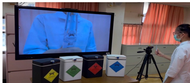
Fig. 5 Medical staff hold the medical waste to the scanning camera to scan the classification marks on the medical waste.
