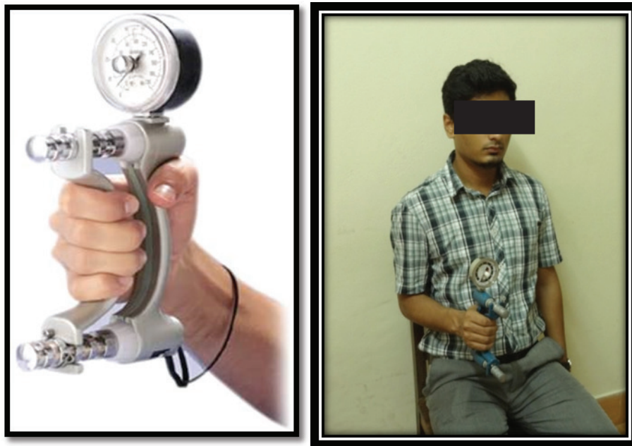
Figure 1: Jamar grip strength dynamometer (Hydraulic Hand Dynamometer, and the position of measurement (A) Jamar dynamometer is set at the level II (B) The subject is in a seated position with the shoulder adducted, not rotated to either side, and the elbow flexed to 90 degrees with the forearm and wrist in neutral position.
