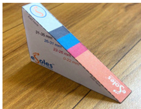
Figure 2: Arch Height Measuring Tool
